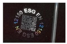
$\hbox{Hi-res LASER marking on tempered glass}$
