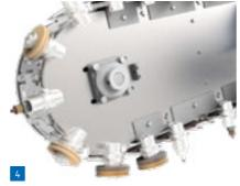
1. High performance spindle 2. Transport system, by means of suction cups 3. Automatic glass measurement 4. 50-fold tool exchanger
