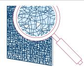
Fracture pattern of toughened glass ESG
