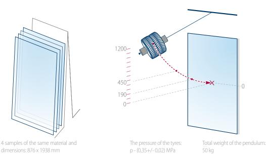
When the tests are performed on asymmetrical materials intended to be fixed in places where there is a risk of hitting from both sides, the test should be performed on both sides
