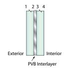
organizations that set standards for safety. Heat-strengthened and tempered glass can be incorporated into laminated glass units to further strengthen the impact resistance. Hurricane resistance, bomb blast protection, UV protection, sound attenuation and ballistic or forced-entry security concerns are all primary uses for laminated glass. For complete industryaccepted information about laminated glass, please review the Glass Association of North America's Laminated Glazing Reference Manual.
