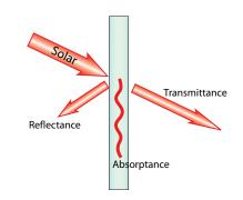
The sum of percent reflectance out + absorptance + transmittance = 100%. An additional consideration is emission, or emissivity. This refers to the reradiation of absorbed energy that can be emitted toward both the exterior and interior of the home. Emissivity is controlled through the use of low-Emissivity, or low-E coatings.
