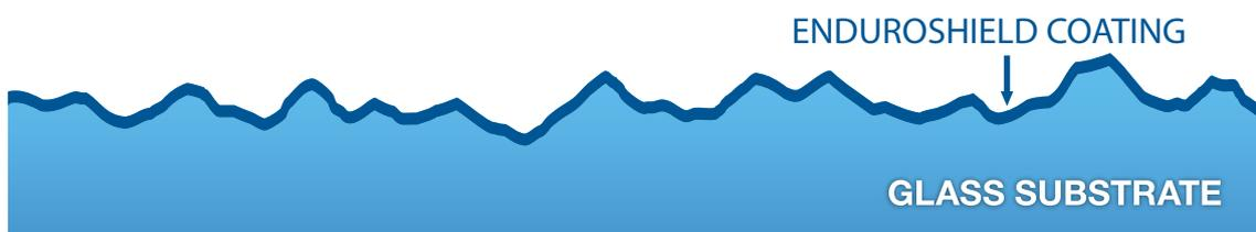
Fig 2. EnduroShield follows the hills and valleys of the glass
