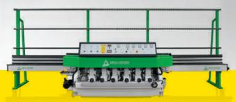
Peripheral straight-line edging machines for processing the pencil edge, OG or flat edge with arris
