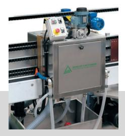
The washing machine applied to the edging machines and bevelling machines outlet conveyor allows the complete cleaning and drying of the processed edges of the glass sheets.
