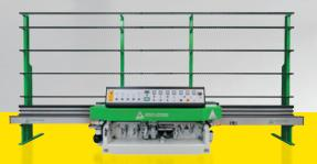
Electronic straight-line edging machines for processing the **flat edge with arris**
