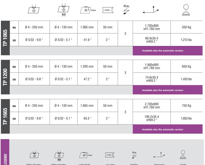
drilling diameter (with 1 head)
