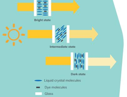
When a low voltage is applied, the dye-doped liquid crystals in the eyrise® cell change orientation and thus regulate the amount of light and heat passing through.
