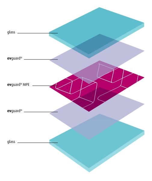
Folienwerk Wolfen GmbH also offers a PET-MPE film ("100 % modified copolyester"). In combination with the **ev**guard®, **ev**guard® MPE establishes an additional advantage in terms of stability, durability, shear modulus effect and printability. **ev**guard® and **ev**guard® MPE can be processed by using the existing suggested cycle times for normal lamination.
