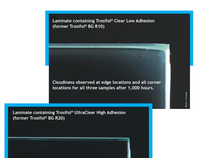
Four glass panels with ground edges were made for each sample type at Trosifol's laboratory in Troisdorf, Germany. Three samples from each sample type were randomly selected for the test, with the fourth being kept for reference.
