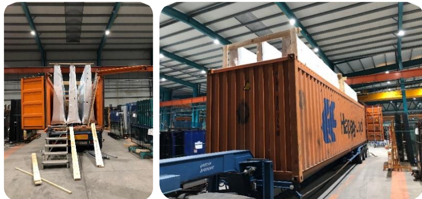
Strapping and full load reinforcement (left) Open top containers (right)
