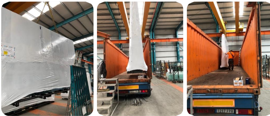
Racks lifted (left) Loading container (center) Loading from outside to inside (right)
