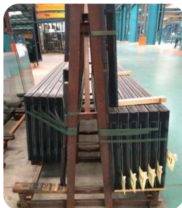
Units strapped together in bundles (left) and units strapped to the rack individually (right)
