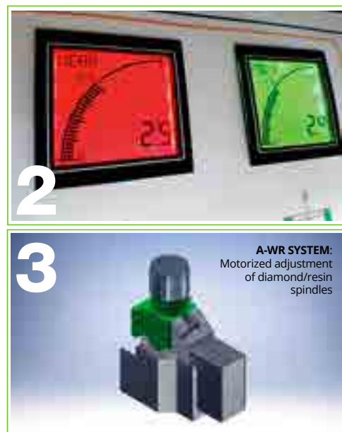
Digital ammeters and polishing wheels automatic wear detection system
