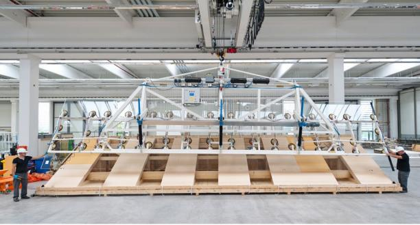
wooden crates with rigid frames | specially designed suction cups
