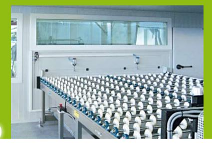
If there is no glass to be washed in the washing machine during the production of laminated glass and insulating glass, the ventilation flaps of the blower close. The result: 25% energy saving.
