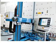
Entry solution for automated insulating glass unit sealing
