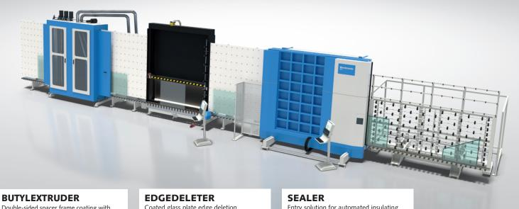
Double-sided spacer frame coating with thermoplastic sealants
