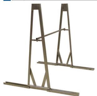
Base arms fold up for ease of shipping and storage whenframes are not in use. 24,000 pound total capacity, 12,000 per side. 60" long x 60" wide x 58" high with 6" spread on top of A. Ships knocked down for lower freight cost.
