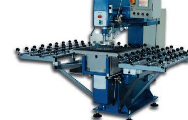
fully automatic glass drilling with ball castor table (accessories)
