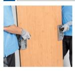
As a new feature, the Bohle Carry Clamp is now equipped with a rubber coating with diamond-shape texture. This coating prevents wet materials from slipping, particularly crafted stone or marble. The transported goods are held safely with two clamps - the heavier the load, the stronger the clamping mechanism.
