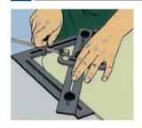
Adjustable angle  $\cdot$  measuring scale on outer edges  $\cdot$  angle made of one piece  $\cdot$  additional scale on straight edge  $\cdot$  centre of circle adjustable to bisecting line
