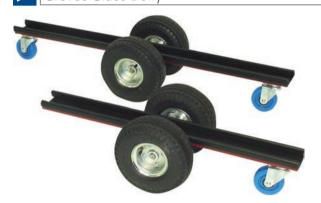
Maneuvers easily indoors and out. 3" (76.2 mm) wide neoprene rubber is easy to clean, prevents slippage and lasts for years. Pneumatic tires reduce breakage caused by vibration. 12" (305 mm) width measured from outside of wheels adds stability. 500 lb. (227 kg) capacity using 8" (203 mm) tires and 3" (76.2 mm) casters.
