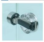
This hinge is a top quality stainless steel hinge for glass-to-glass mounting. This hinge is suitable for inset doors. It is adjustable in three dimensions and has a snap-on function for easy mounting and dismounting. It is equipped with a self-closing spring mechanism and is well suited for use with dampers BO 55 002 30/31 and BO 55 002 35/36.
