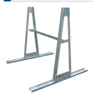
Heavy duty, 146 lb. Steel A-Frame Rack. 24,000 lbs. capacity, 12,000 lbs. per side. Ships knocked down for lower freight cost. Bottom U-channel is 4" wide with 1" side ledges and is designed to hold wood 2 x 4's to support the load. Customer furnishes the wood. Glass sheet width depending on customer requirements. Glass height not to exceed 12" above product height. Not to exceed max. weight capacity.
