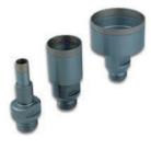
Drill Speeds: ø 3-4 mm = 4000-5000 rpm ø 5-15 mm = 2000-3000 rpm ø 16-25 mm = 1500-2000 rpm ø 26-50 mm = 500-1500 rpm ø 51-100 mm = 300-800 rpm For float glass fabrication use · drill base made of steel · covered with protective lacquer · diamond coating from sintered material · drill hasto be sharpened before first use - in 75mm and 95mm lengths (Forvet machines) available
