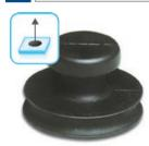
The Veribor<sup>®</sup> all-rubber vacuum lifter ideally lends itself to lifting and carrying ifferent loads. It is suitable for holding smaller objects or for opening the covers of cable ducts. The vacuum is generated by simply pressing the suction pad onto the respective surface, which enables quick and efficient working. The lifter can be loosened from the surface by slightly lifting the release nipples laterally.
