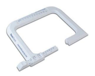
GlassCheck is used for measuring the overall glass thickness of already installed glass panes and insulated glass. The device is suitable for measuring glass thicknesses of up to 4 3/4" (120 mm). The device also features an integrated glass thickness gauge which offers the possibility of determining the thickness of single glass panes from 1/16" - 1" (2 - 25 mm).
