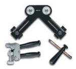
Corner cut-outs can be produced quickly and effortlessly  $\cdot$  no more troublesome drilling or sawing  $\cdot$  reduces workload e.g. when producing tempered glass  $\cdot$  for manual corner cutting in flat glass  $\cdot$  comes in a practical storage case
