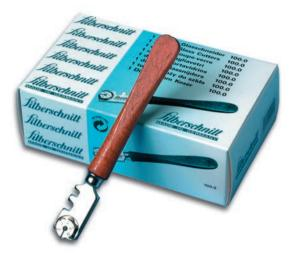
Six cutting wheels made of alloyed steel and tempered by a patented method guarantee high cutting quality and long service life. Turrets and cutting heads are nickel-plated. An oil-soaked felt ring supplies lubrication for wheels and axles. The handle is produced exclusively from ecologically controlled and approved varieties of wood. The Silberschnitt<sup>®</sup> glass cutters are particularly economical because wheels and turrets are replaceable. This cutter is suitable for general cutting.
