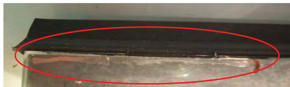
Figure 11 - Delamination on sample 44.2-LA-E/05, after 7 weeks UV irradiation test
