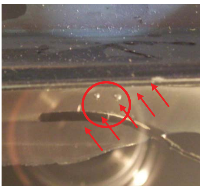
Figure 5: Defects recorded after 21 weeks at 60°C: a) bubbles in sample 44.2-HA-E/01; b) bubbles in sample 44.2-HA-E/03
