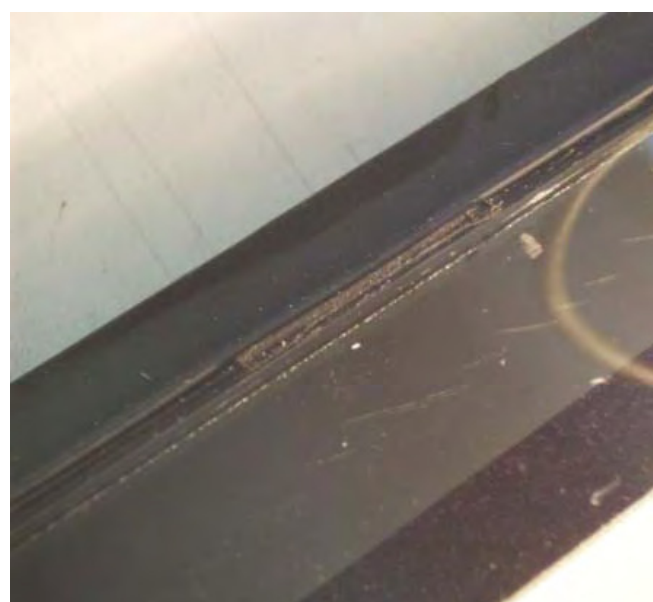
Figure 5: Defects recorded after 21 weeks at 60°C: a) bubbles in sample 44.2-HA-E/01; b) bubbles in sample 44.2-HA-E/03
