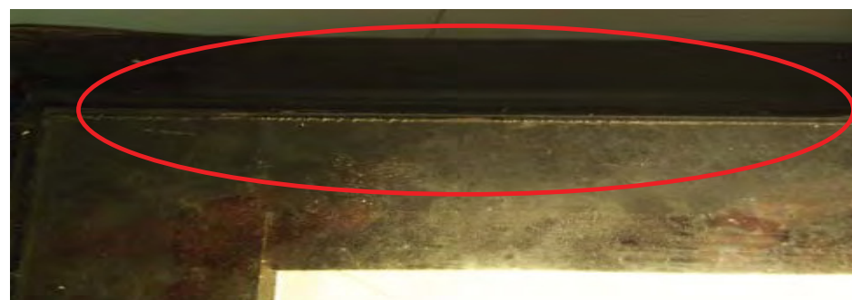
Figure 12 - Bubbles on sample 44.2-LA-E/05, after 7 weeks UV irradiation test
