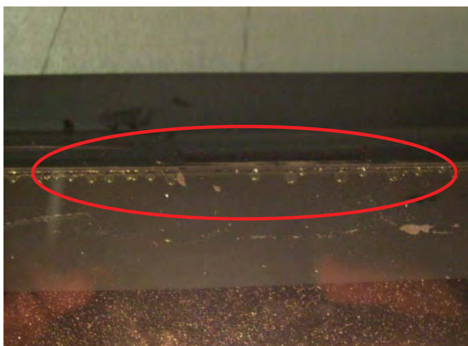
Figure 10 - Bubbles in sample 44.2-HA-C/07, after 7 weeks UV irradiation test
