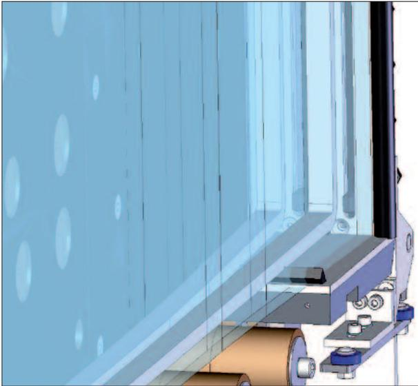
Filling the triple insulating glass unit with inert gas
