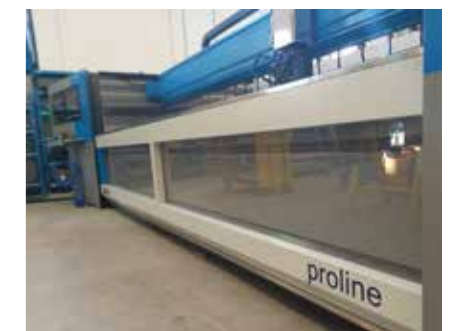
Front and rear hatch with pneumatic movement to better protect the cutting area and reduce the dispersion of water and abrasive material
