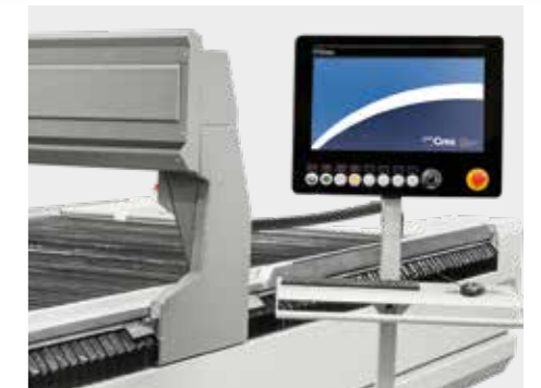
Console on a mobile trolley with 21.5" touch screen (optional)
